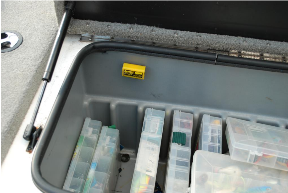
Picture 14 - Tackle storage protected by vapor capsules Vapor capsule inside tackle box and one outside
