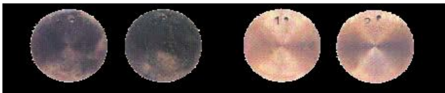
Picture 4 - Tarnish on copper (left) and bright copper (right)
